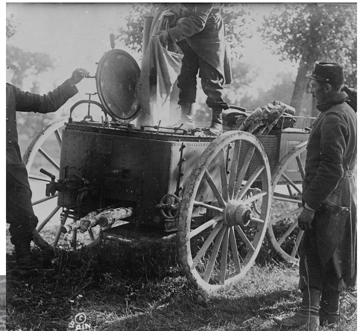
Above: Cooking for French Soldiers during battle. One of the few photos available which shows how the fuel (in this case wood) went into the vehicle. In their way, cookers changed the world culture as, for many men, it was the first time they learned to cook. Part of the George Grantham Bain Collection (Library of Congress).
